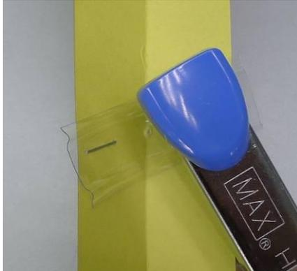
Staple the reinforcement part with two staples.
