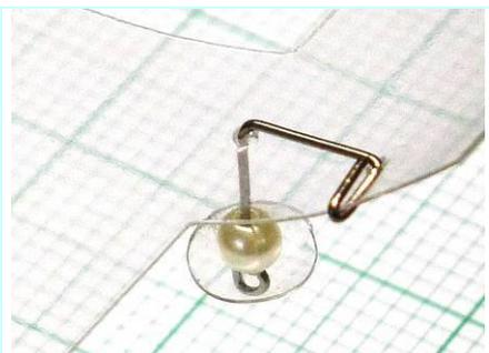
Using pliers, fold the end of the wire like the picture above to fix the axis part onto the blade.
